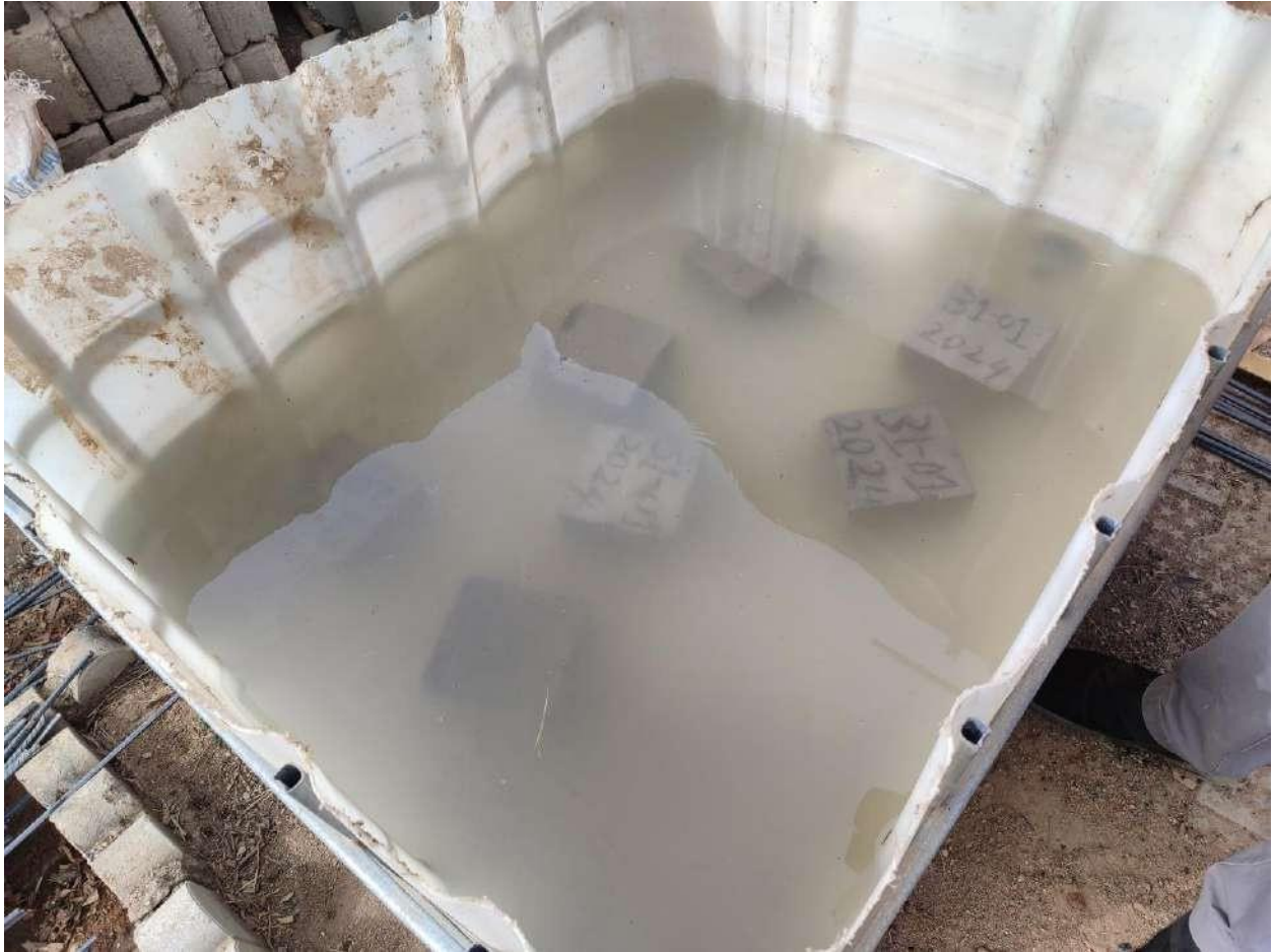
Curing of cubes for testing
