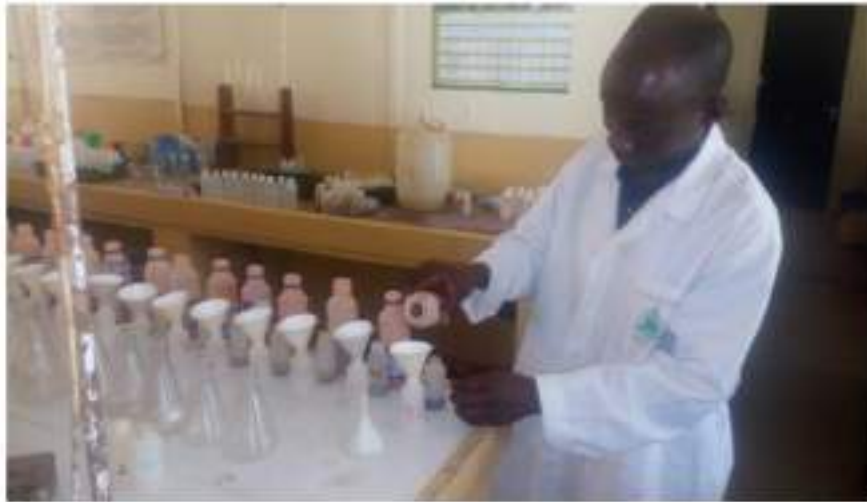
Plate 1: Photograph representation of sample filtration for Atomic Adsorption Spectrometer
